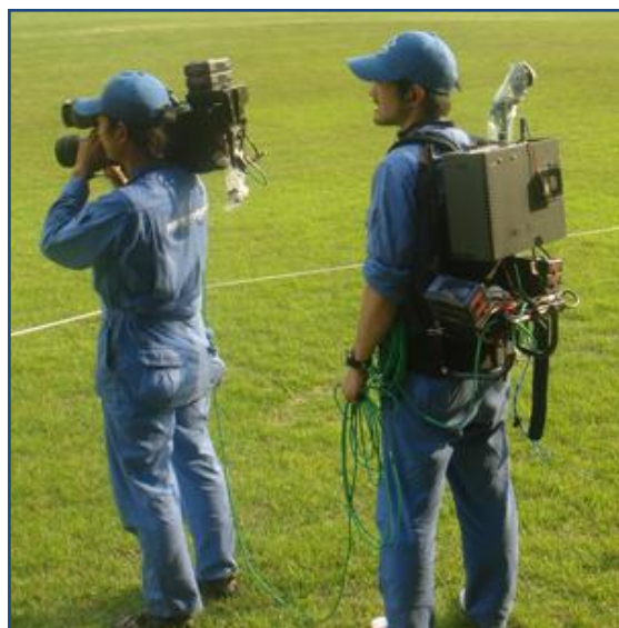
The ultra-compact HD c3000e can be integrated with an HD camera using a commercial V-shaped holder.
